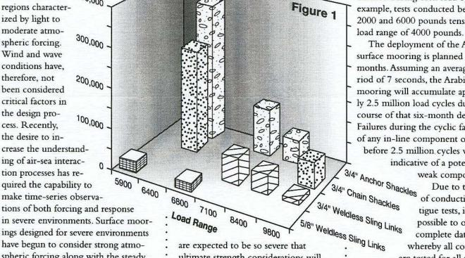
ultimate strength considerations will be superseded by the fatigue properties of the standard hardware components.
