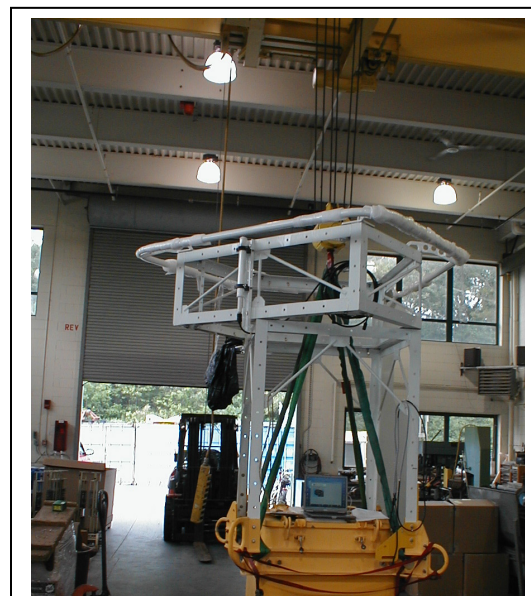
Fig. 3: Rigging of the assembled buoy for buoy spin (or ‘hard-iron calibration’).
