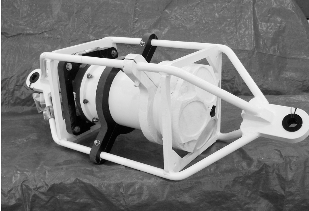
Figure 8. Photograph of the 300-kHz ADCP in welded aluminum load cage. Anti-fouling paint has been applied to the ADCP transducer head.
