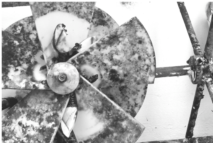
Figure 38. NTAS-2 VMCM rotor after recovery.
