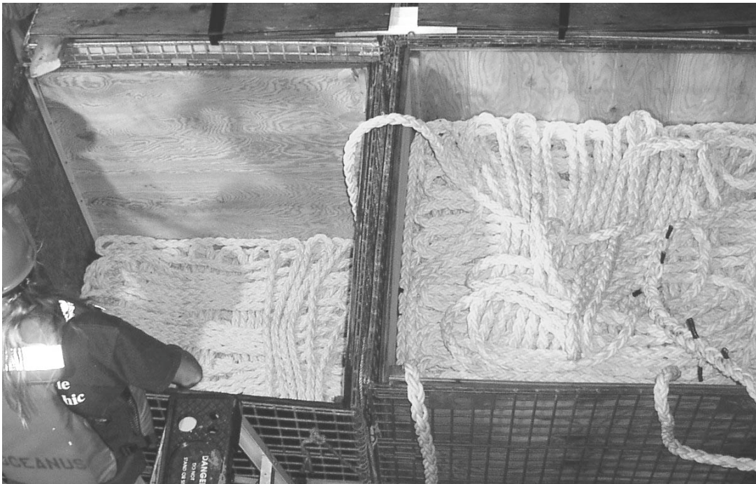
Figure 19. Polypropylene line faked out in wire baskets during deployment.
