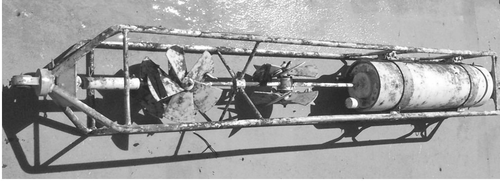
Figure 37. NTAS-2 VMCM after recovery.
