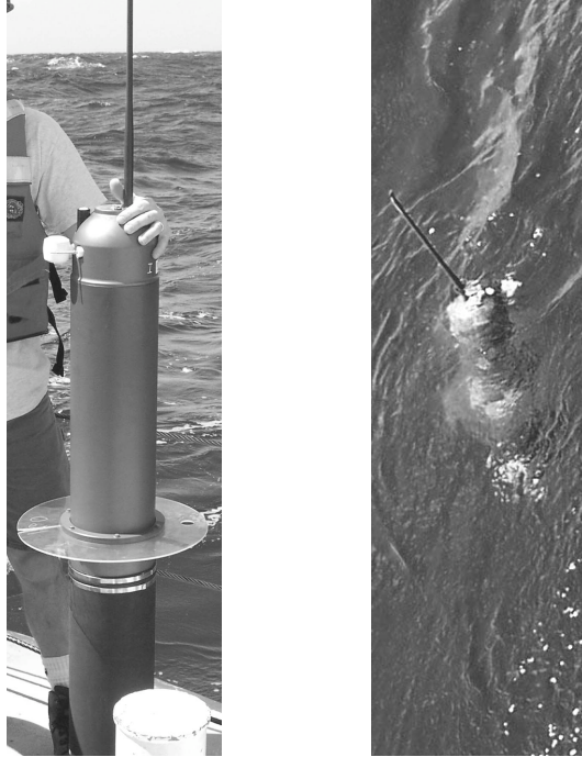
Figure 31. SOLO float on the stern prior to launch (left) and in the water just prior to submersion (right).
