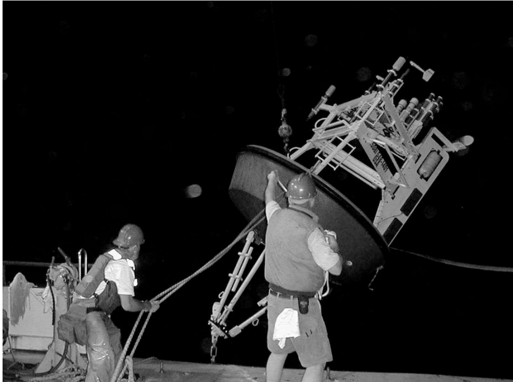
Figure 18. Deployment of the NTAS-3 disc buoy. The three lines visible are (clockwise from right) outboard deck bail slip line, quick-release trip line, and inboard deck bail slip line. The bridle slip line has already been removed.
