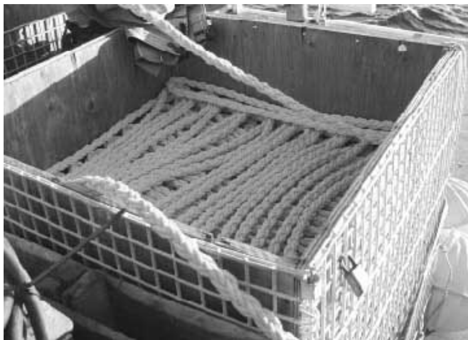
Figure 19. Polypropylene line faked out in wire basket ready for deployment.
