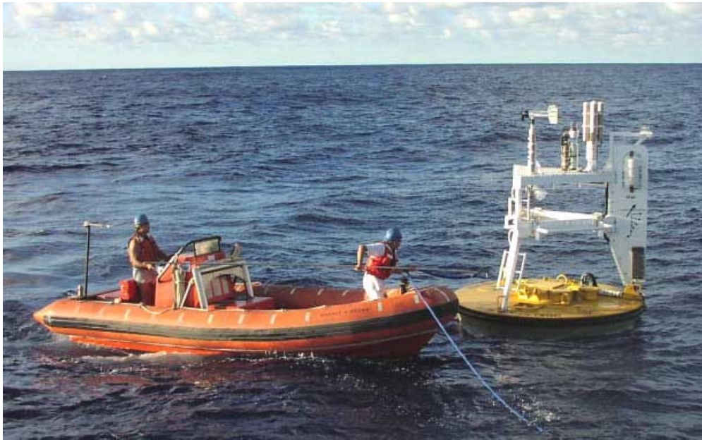
Figure 30. NTAS-1 buoy hook-up operation. The small boat maneuvered into position so that a lifting pennant and hauling line could be attached to the buoy deck bail by means of a specially designed pick-up hook.
