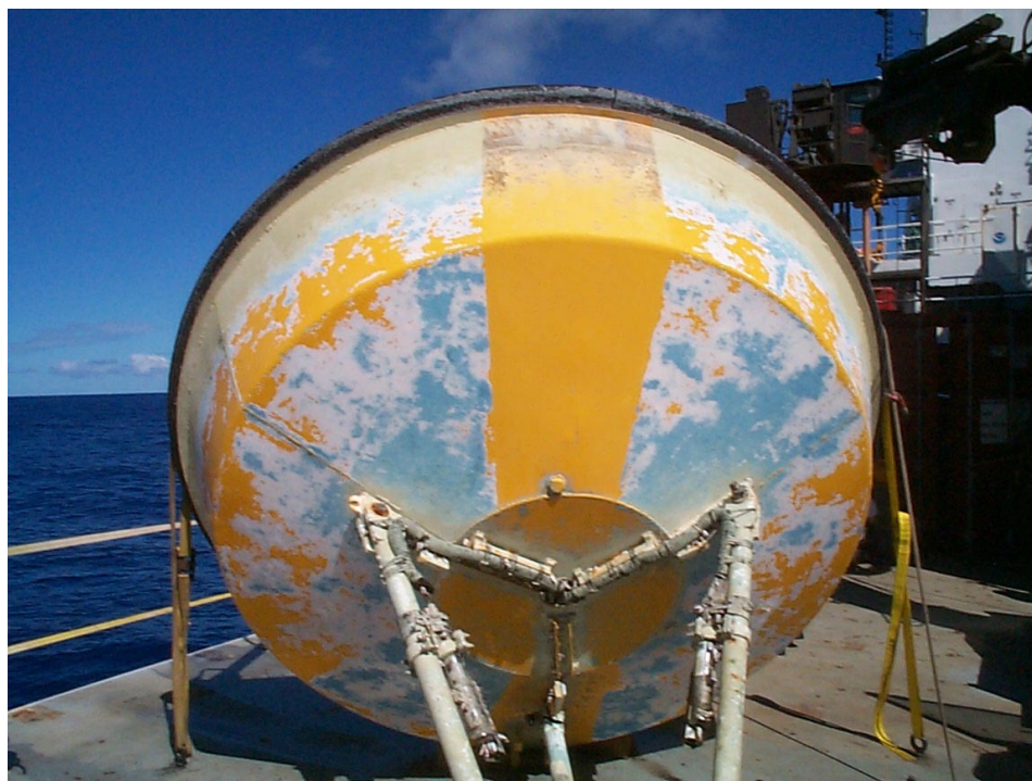
Figure 34. NTAS-1 discus buoy hull after recovery.
