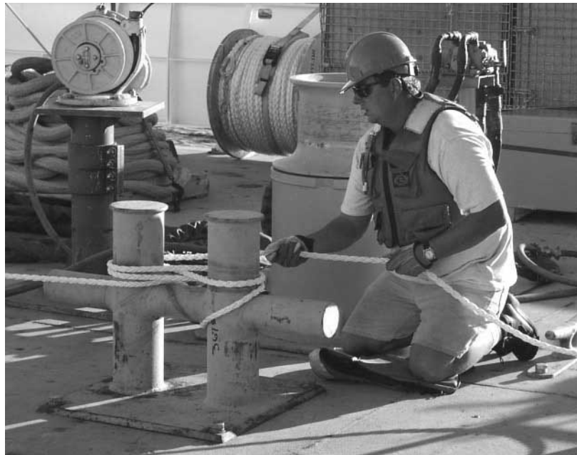
Figure 22. Position of line handler during payout of synthetic line through the H-bit.
