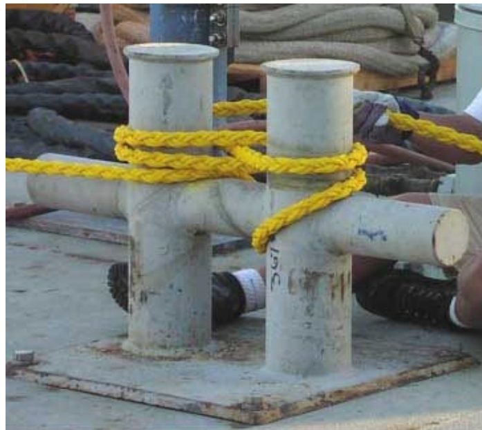
Figure 21. Polypropylene line and H-bit during manual payout.
