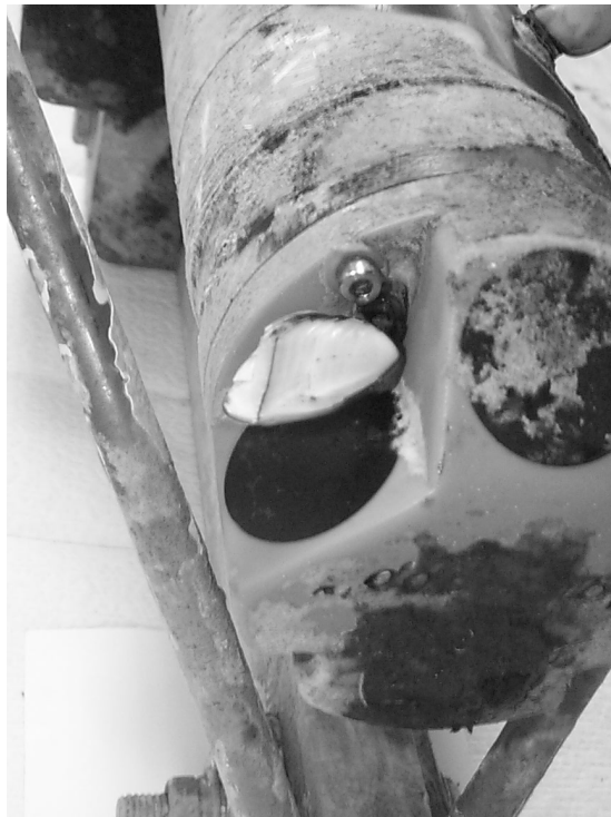
Figure 38. Fouling on the Aquadopp current meter.
