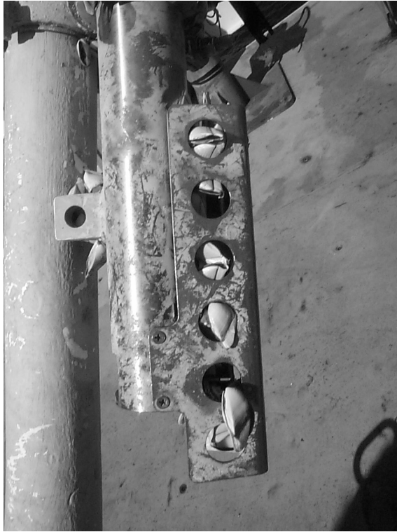
Figure 37. Gooseneck barnacle fouling of MicroCAT sensor area.
