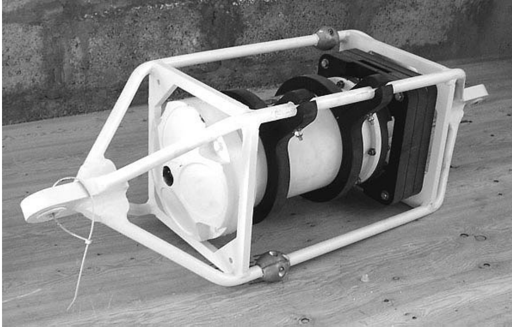
Figure 6. Photograph of the 300-kHz ADCP in welded aluminum load cage.
