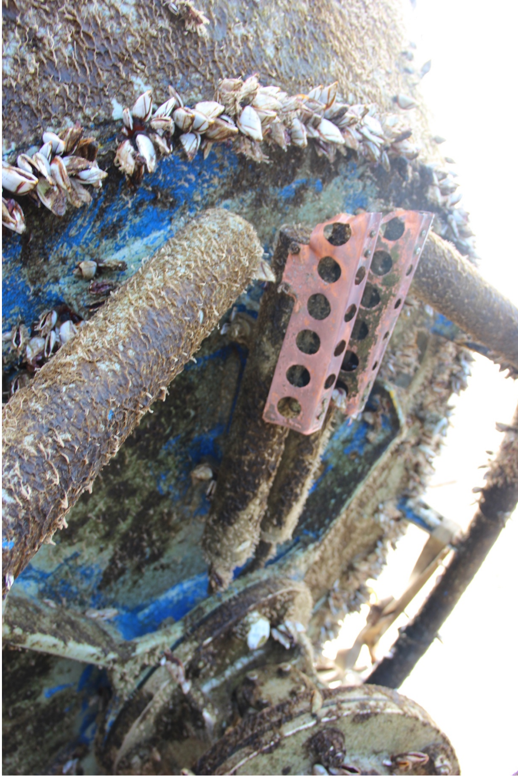
Figure IV-6. . NTAS 17 buoy bridle's instrumentation at recovery.
