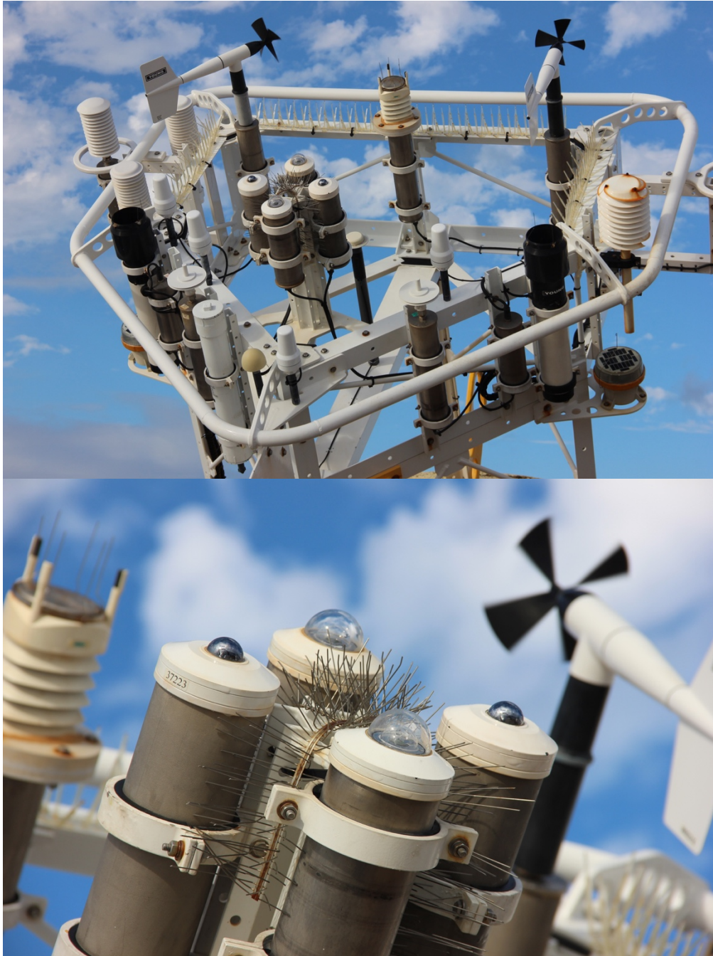
Figure IV-3. ASIMET meteorological sensors immediately following recovery of NTAS17.
