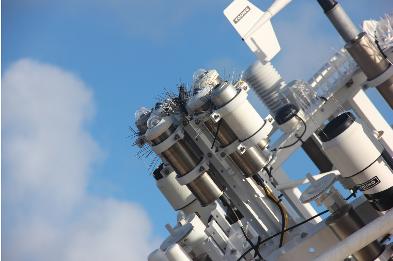
Figure III-4. Closeup of ASIMET radiation sensors on NTAS 18 prior to deployment.
