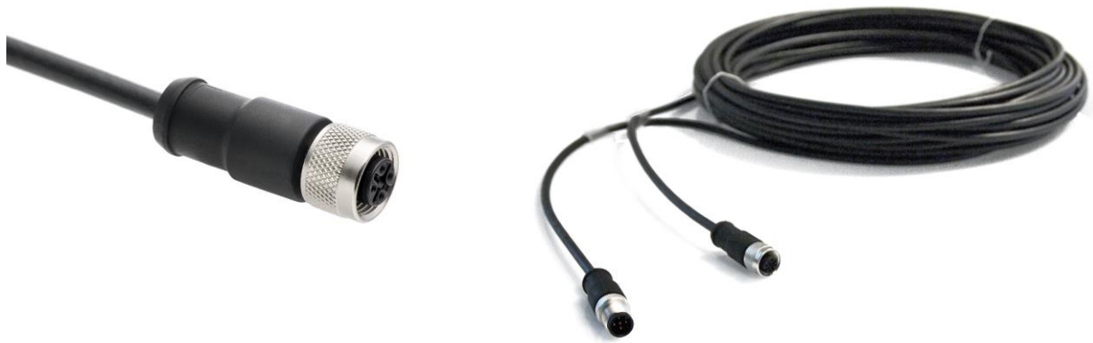
Figure 0.7 On the left the SR30-D1 cable with M12-A female connector on sensor end, pigtails of 0.15 m and conductors with ferrules. Its length is 5 metres standard and available in 10 and 20 metres too. On the right the optional Hukseflux extension cable with connector pairs, with male and female M12-A connectors, available in 20 metres
