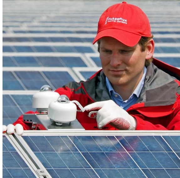
Figure 0.3 Two SR30-D1 secondary standard pyranometers with digital output for GHI (global horizontal irradiance) and POA (plane of array) measurement applications
