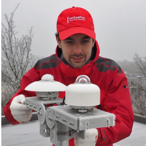
Figure 0.2 Dew deposition and frost (as in the photo): clear difference between a non-heated pyranometer (back) and SR30-D1 with RVH™ technology (front )
