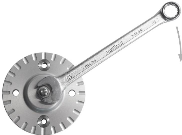
Figure 6.3.1.3 SR30-D1 levelling mount seen from above: (un)locking with a 10 mm spanner
