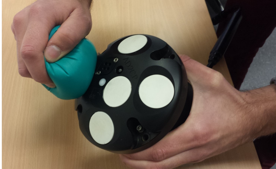
Figure 7. Example of an amplitude test. Covering one beam at a time with a water filled glove.
