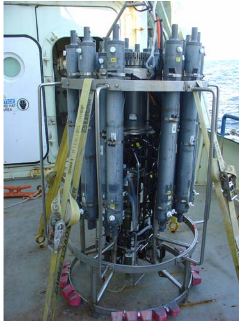
Figure 6.3: Climode CTD/Rosette on board Oceanus voyage 434.
