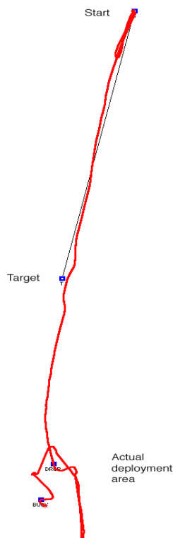
Figure 2.6: The track of RV Oceanus during the deployment of mooring F and during the subsequent survey of the anchor position. The anchor drop and buoy positions are indicated by blue squares (see next figure for details).
