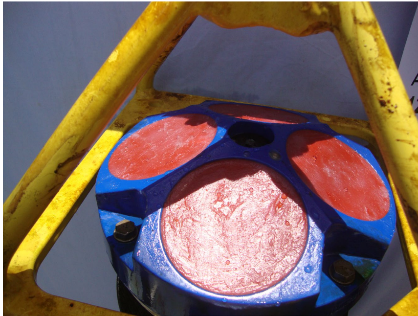
Figure 5-2. WHOTS-7 300 kHz ADCP deployed at 125 m after recovery.
