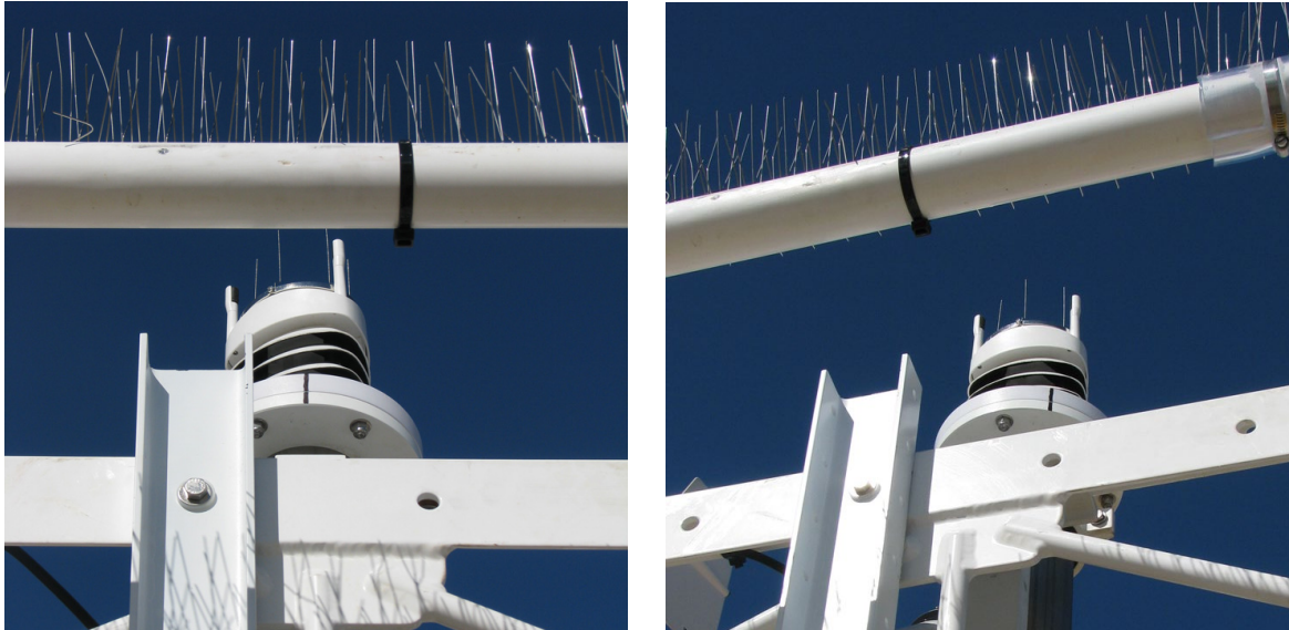
Fig 2-3: Orientation of Vaisala WXT-520 before (left) and after (right) rotation.
