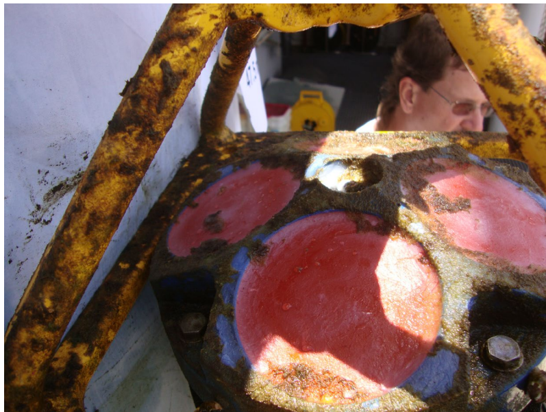
Figure 5-3. WHOTS-7 600 kHz ADCP deployed at 47.5 m after recovery.
