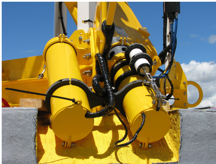
Fig. 3-2. Remote line deployment system on the WHOTS-8 buoy.
