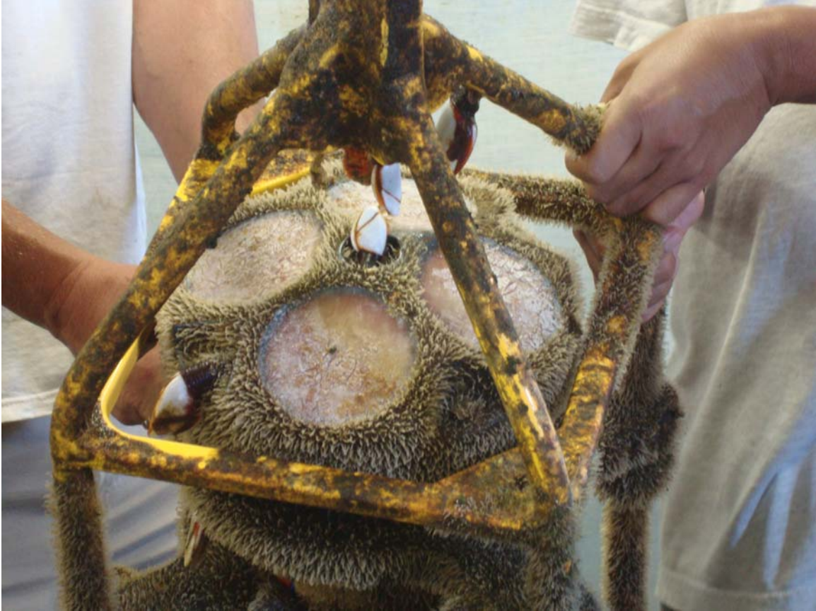
Figure 5-3: WHOTS-6 ADCP deployed at 47.5 m after recovery.
