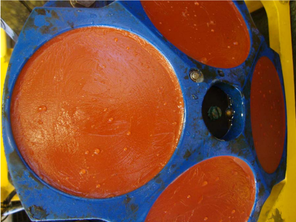
Figure 5-2: WHOTS-6 ADCP deployed at 125 m after recovery.
