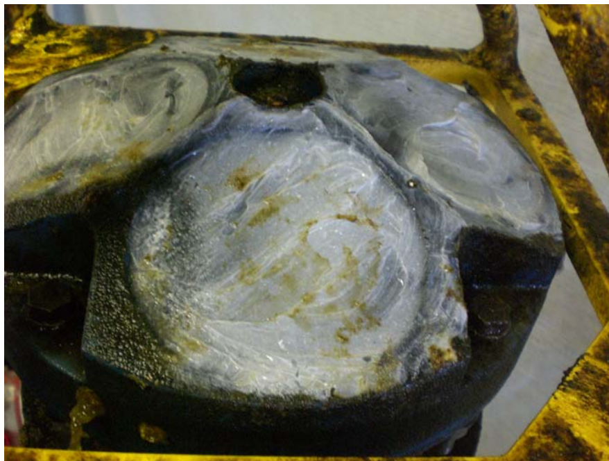
Figure 5-3: WHOTS-4 ADCP deployed at 48.5 m after recovery.
