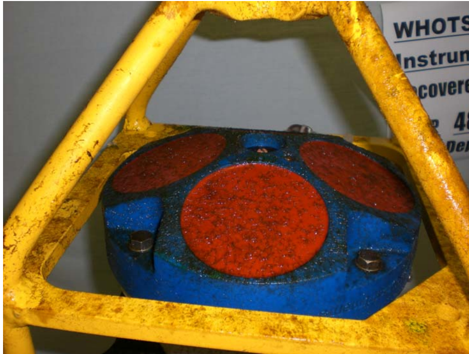
Figure 5-2: WHOTS-4 ADCP deployed at 125 m after recovery.
