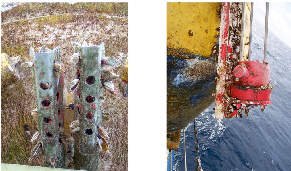
**Figure 38. WHOTS-1 buoy instrumentation: MicroCATs (left) and surface-following temperature sensor (right).**
