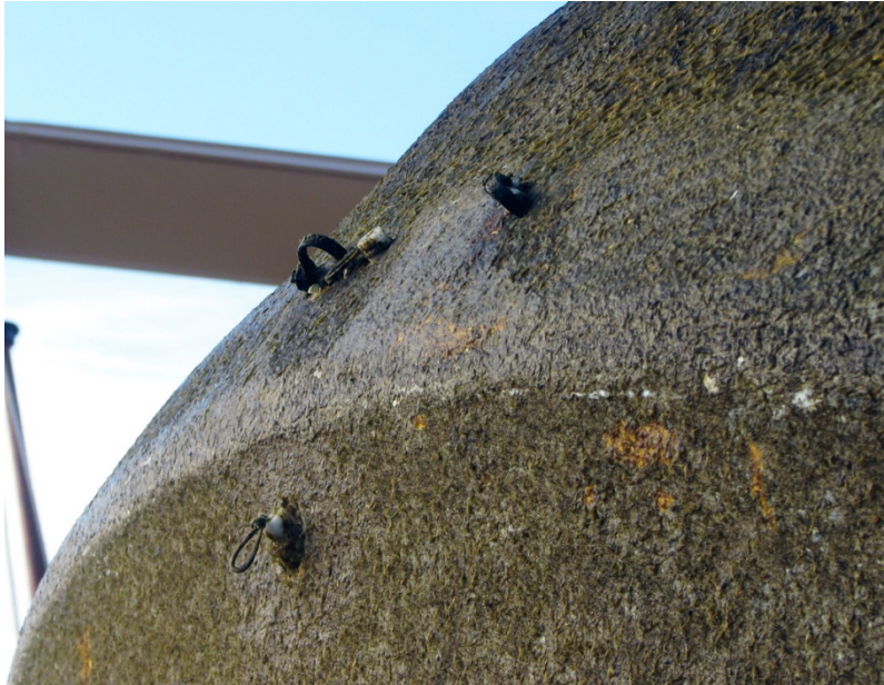
Figure E1. WHOTS-9 buoy hull SST instruments.
