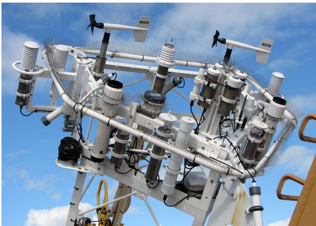
Figure 7. WHOTS-10 tower top, showing the location of ASIMET modules. A SBE-39 (port side inboard of the HRH module) supplemented the ASIMET air temperature measurement. A Vaisala WXT multi-parameter sensor was mounted between the two WND modules. A self-contained GPS module was mounted just aft of the port BPR.
