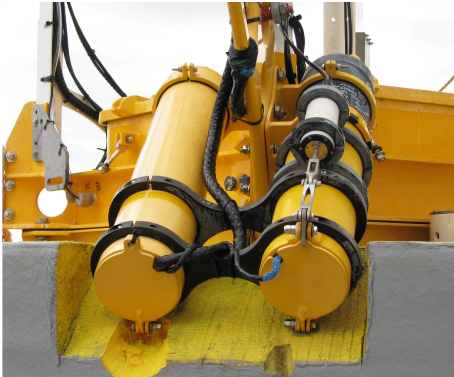
Figure 6. Remote line deployment system on the WHOTS-10 buoy.
