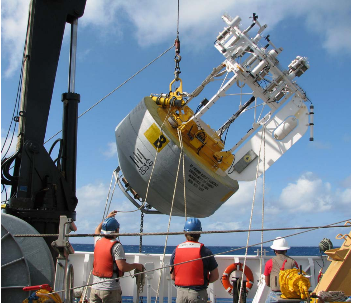
Figure 10. WHOTS-10 buoy deployment. The buoy is lifted over the (non-removable) gunwales with the ship's crane. Tag lines for the crane whip, quick release, buoy deck, and buoy tower can be seen.
