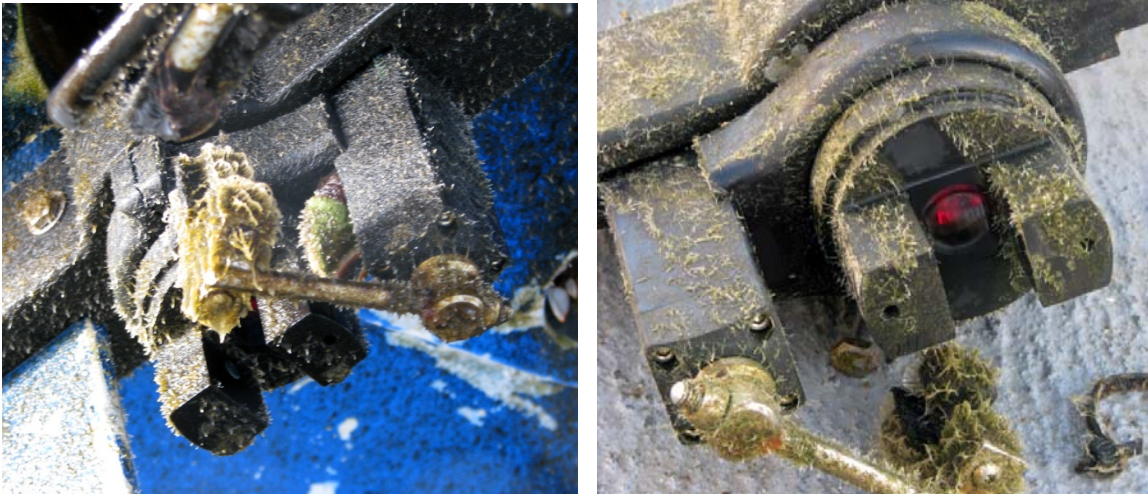
Figure E5. Sensor end of chlorophyll fluorometer (left) and close up of optical window (right).
