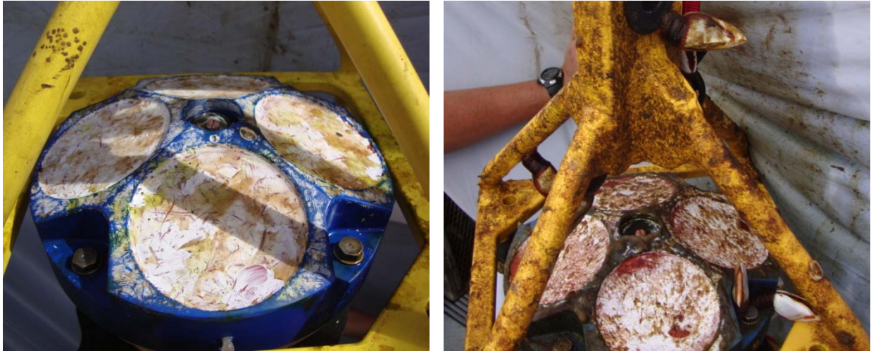
Figure C1. WHOTS-9 ADCPs deployed at 125 m (left) and 47.5 m (right) after recovery.
