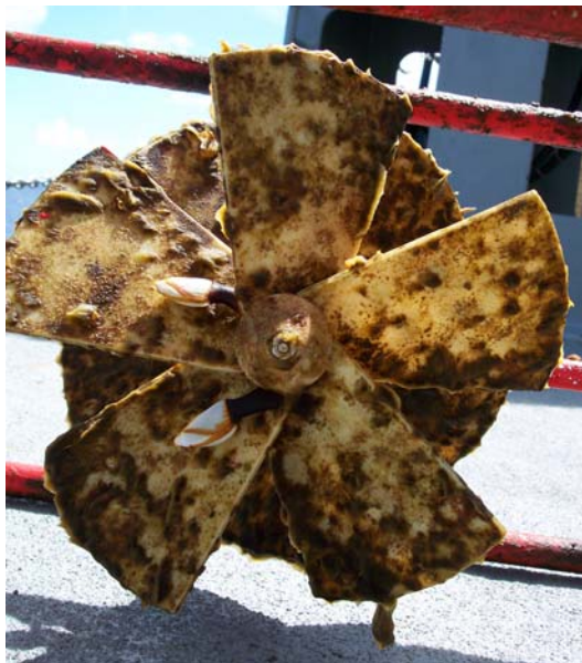
Figure 1. Close-up of fouling present on NGVM 012 after recovery.
