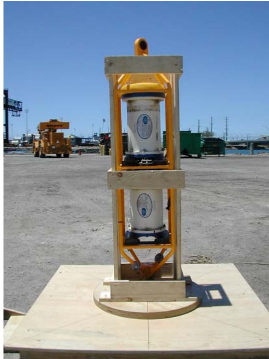
Figure 5-25 Turntable used to test the performance of the internal compass of the ADCP SN4891 with external battery module installed.
