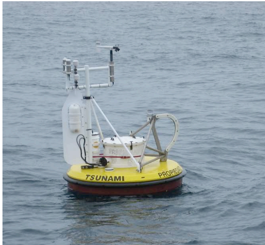
Figure VI.C.2. DART II surface mooring with its reduced set of IMET sensors.
