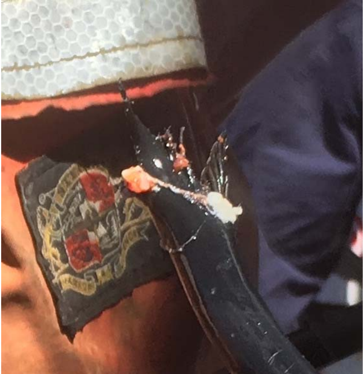
Figure IV-2. Broken 3/8" wire somewhere on the second 500 m wire shot on Stratus 16.
