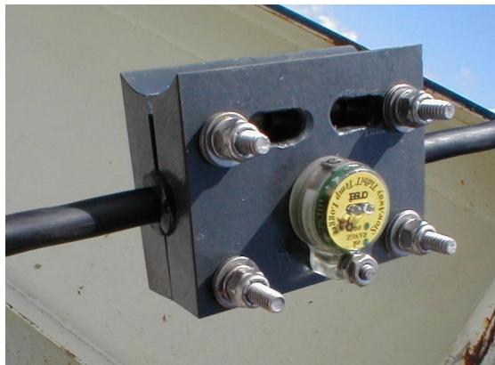
Figure 8: Photograph of Tidbit temperature logger attached to wire-rope mounting bracket.
