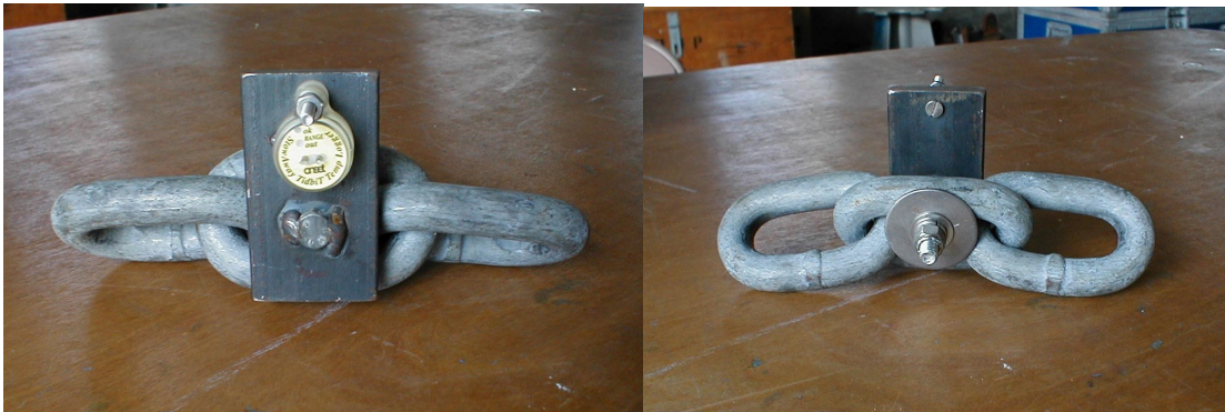
Figure 7: Photographs of Tidbit temperature logger attached to chain mounting bracket. Left, front view; right, back view.
