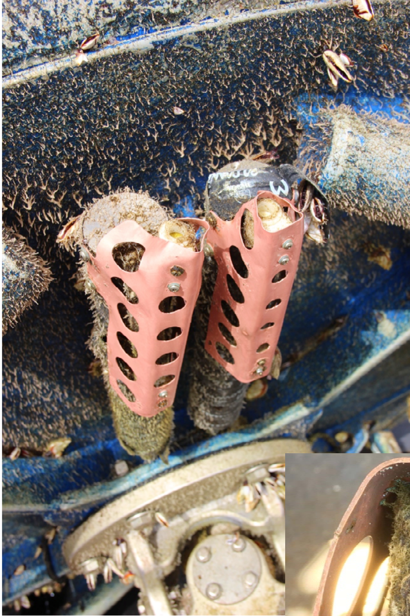
Left: SST sensors on bridle. Below: SBE 37 at 40 m (SN 684) with missing poison plugs.
