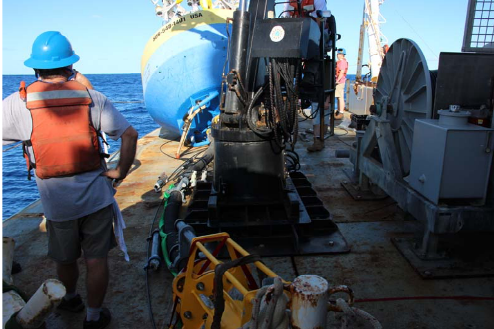
Figure IV-5. Picture of instruments (current meter and SBE 39) clamped to compliance section prior to deployment of NTAS-14 on December 13 2014.
