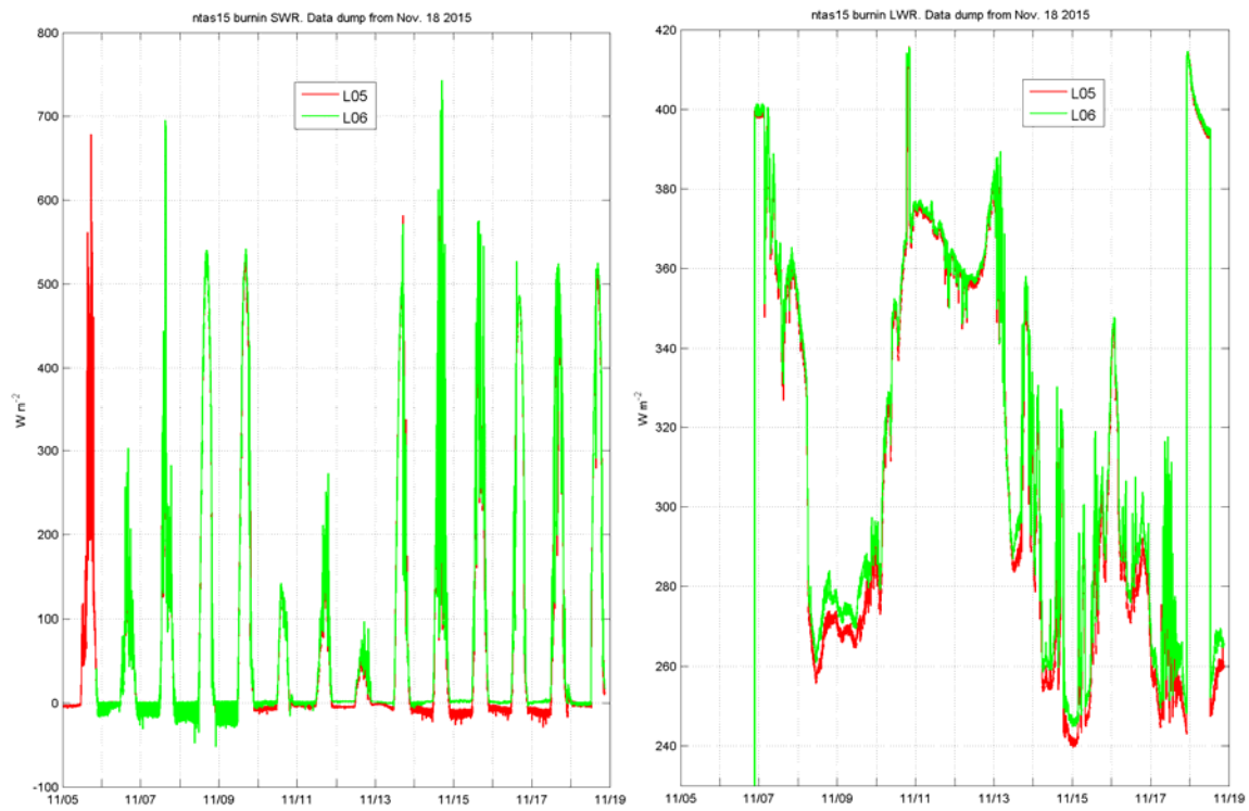
Figure II-5. NTAS-15 burn-in: downwelling radiation, shortwave SWR (left) and longwave LWR (right).
