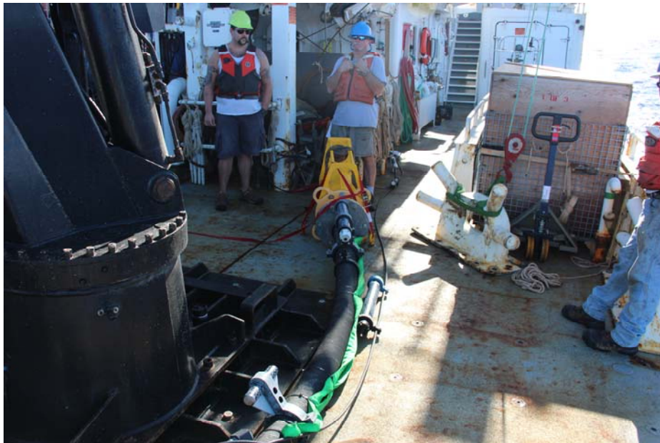
Figure IV-4. Picture of instruments (current meter and SBE 39) clamped to compliance section prior to deployment of NTAS-14 on December 13 2014.
