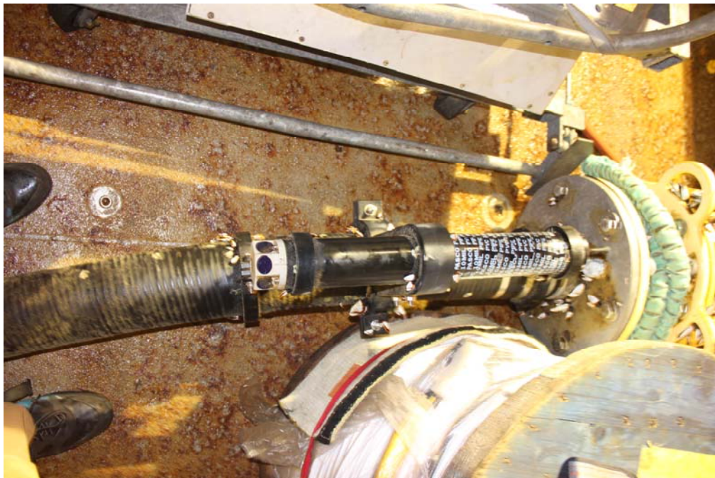
Figure IV-6. Picture of current meter clamped to bottom of compliance section on NTAS-14 during its recovery on February 4 2016.
